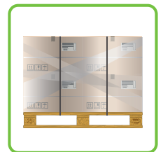
A correctly loaded pallet
