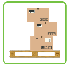
An incorrectly loaded pallet
